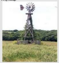
A windmill will pump water from stormwater ponds to prevent stagnation
